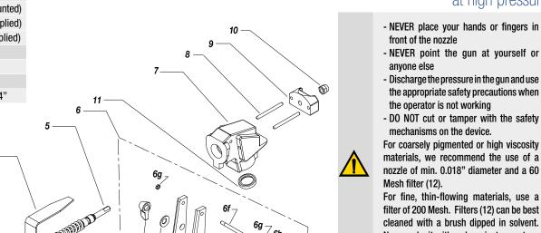
nozzle of min. 0.018" diameter and a 60 For fine, thin-flowing materials, use a filter of 200 Mesh. Filters (12) can be best
